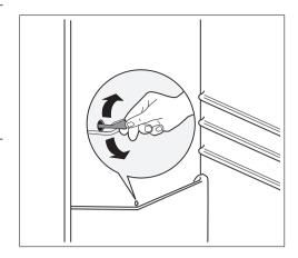
It is important to periodically clean the defrost water drain hole in the middle of the refrigerator compartment channel to prevent the water overflowing and dripping onto the food inside. Use the special cleaner provided, which you will find already inserted into the drain hole.
